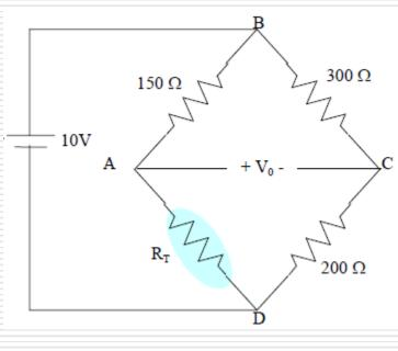
A thermistor is placed in 100 °C environment, and its measured resistance is 20 KΩ; the thermal constant is β=3650. If the thermistor is used to measure a particular temperature; and its resistance is measured as 500 KΩ, determine the thermistor temperature.
