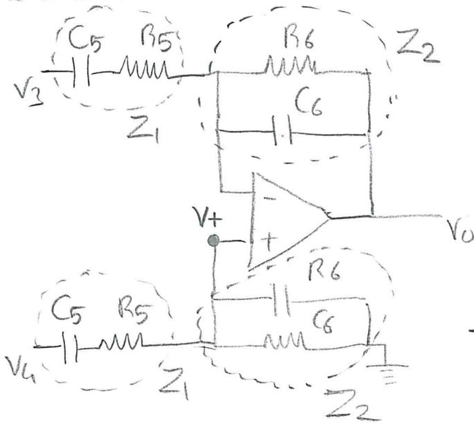
$$V_+ = \frac{V_4 \cdot Z_2}{Z_1 + Z_2}$$
