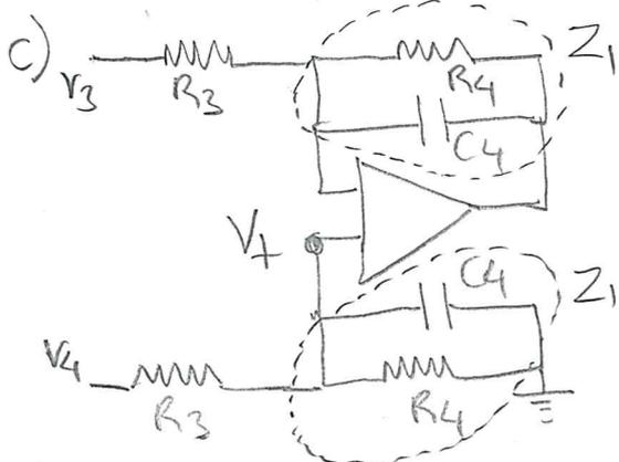
$$\frac{V_4}{R_3 + Z_1} \cdot Z_1 = V^+ \quad \frac{V_3 - V^+}{R_3} = \frac{V^+ - V_b}{Z_1}$$
