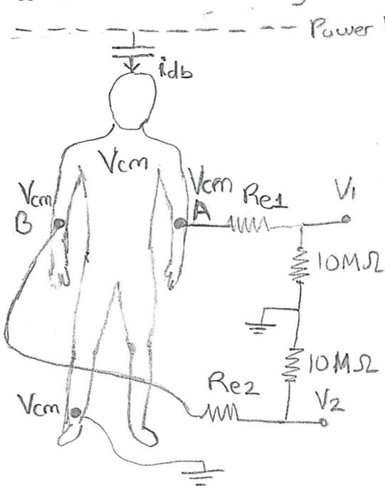
tes noise in two ways, in common mode and in differential mode. As  $V_{cm}$  is the same at inputs A and B, instrumentation amplifier operates in common mode and  $V_{cm}$  is multiplied with common mode gain  $A_c$  and appears at output
