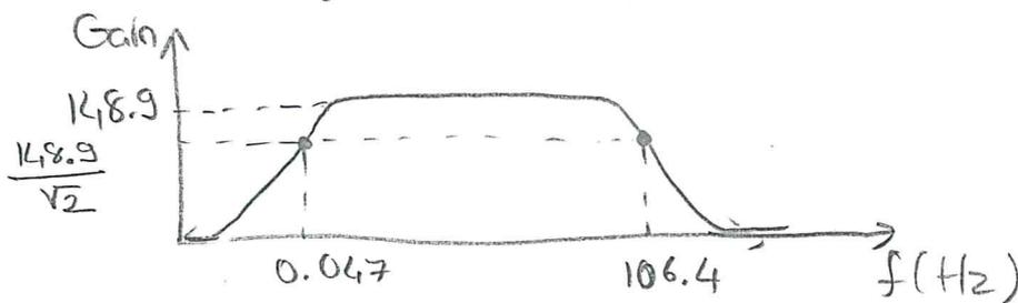
b) The differential gain of the the circuit at 50Hz is 148.9 since this frequency is at the passband region. CMRR of this circuit at 50Hz is given as
