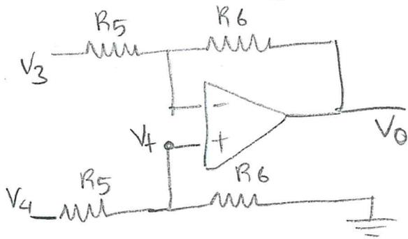
$$V_4 = \frac{V_4 R_6}{R_5 + R_6}, \quad \frac{V_3 - V_4}{R_5} = \frac{V_4 - V_0}{R_6}$$
